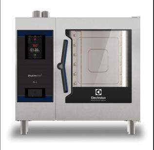
219606 (ECOE61K3L30) SkyLine ProS Combi Boilerless Oven with touch screen control, 6x1/1GN, electric, 2 cooking modes (recipe program, manual), automatic cleaning, spray gun, 6-sensor probe, 3-glass door and IoT module- 208V US
